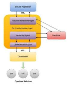
Fig. 5. Communication Mechanism between the Service Abstraction Layer and the Orchestrator
